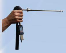
The Sample Conditioning Unit is mounted directly at the sampling probe exit, where excess moisture rapidly condenses and separates from the gas sample. This minimizes contact of the gases with moisture, which could potentially affect NOx and SO2 measurements.
