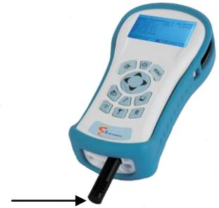
1. Push the **On/Off** power button to activate the monitor & sampling pump.
