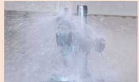
Rated to IP66 water- and dust-proofing standard and oil resistance improved.
