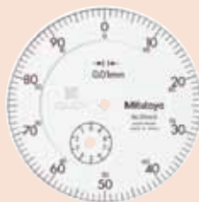
Continuous dial (Bi-directional graduation)
