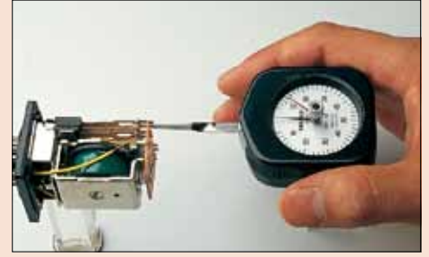
Measuring contact force on a relay.
