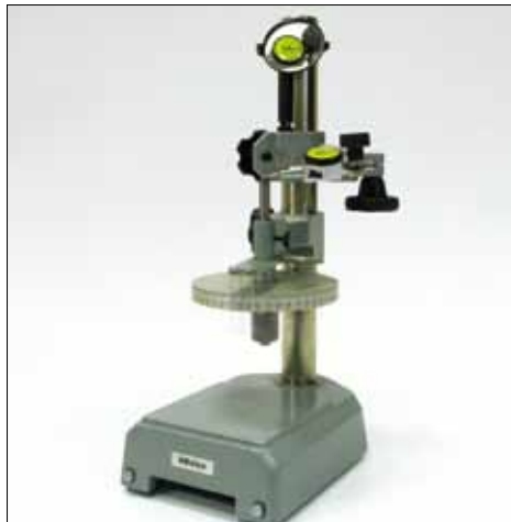
Calibrating a lever indicator.
