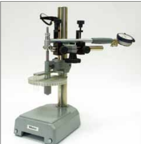
Calibrating a bore gauge.
