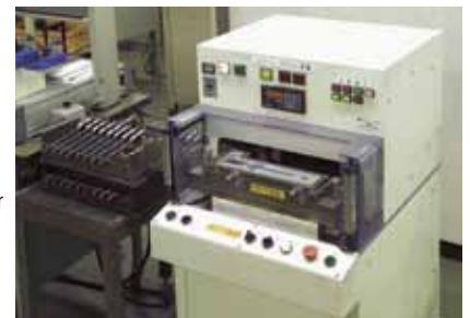
Air leak test equipment for coolant proof caliper
