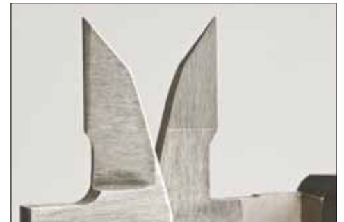
Carbide-tipped jaws for inside measurement
